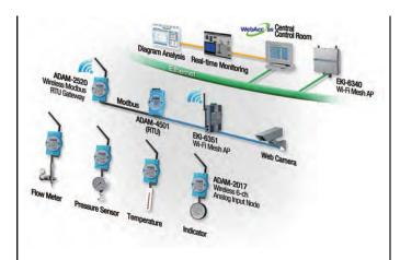
effects. OnsiteRTU module (ADAM-4501), supports Modbus RTU/TCP, completes onsitedata acquisition, packaging and uploads. Through an industrial wirelessnetwork, built by EKI-6351 and EKI-6341 modules, remote WebAccesssoftware compiles and analyzes the data of well mouths. WebAccess? B/Sstructure shows its outstanding performance when it comes to remotemanagement and maintenance.
