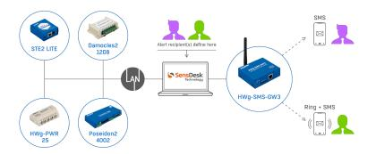
However, both options (SMS-GW unit / SMS alerting from the Portal) have their limitations and advantages. Using gateway unit only can cause a situation, when the monitoring device is turned off (disconnected) - sending a critical alert message or making a call won't be available. So the combination with the Portal makes alerting even more reliable.
