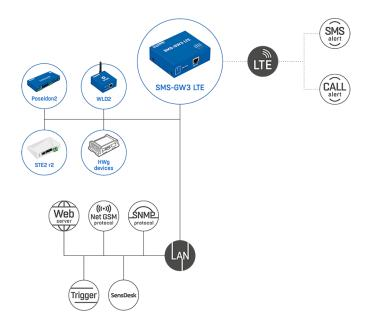
Both 2G (GSM) and LTE (nowadays it's probably not necessary to explain the difference between wireless broadband standards) SMS gateways, named SMS-GW3 as it is the third version of the gateway from our production, serve the same function - to send an alert in the form of a user/device-defined SMS message or to make a call-out alert - which is basically a call to a target phone number.
