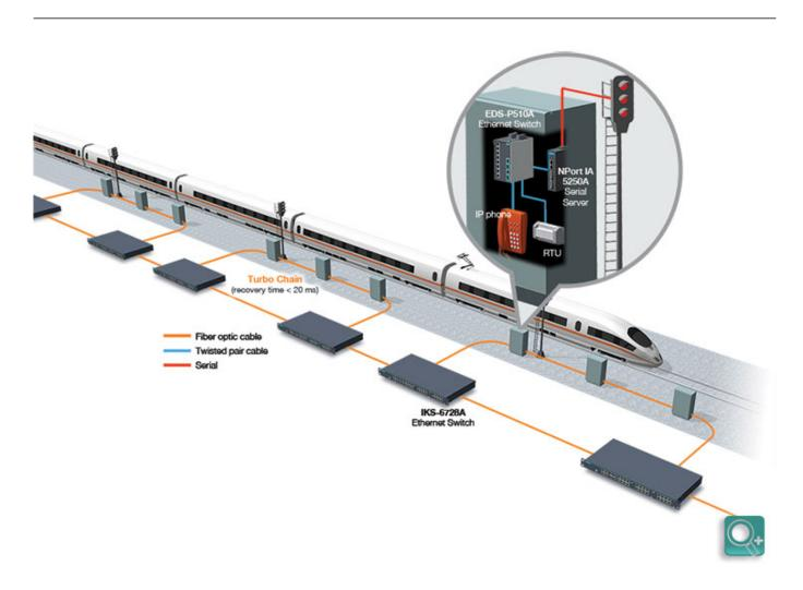
**EN 50121 Railway Communication Network for Mainline Signaling and Train Control Applications**
